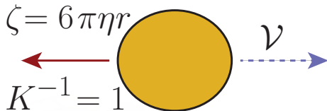
Figure : The drag on a spherical body of radius r moving through a fluid of viscosity \eta at low Reynolds numbers (small speed v ) has a friction coefficient that obeys Stokes' law \zeta = 6\pi\eta r .
