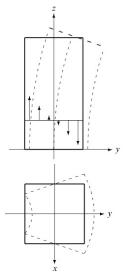
N.B.: form of u<sub>v</sub> is determined by shear free conditions
